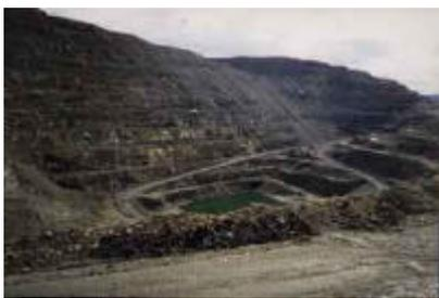
Figure 32: Medvezhka mine, south of Noril'sk. An example of extensive surface nickel and copper mining. Nowadays almost completely replaced by underground mining. Photo taken by Olga Tutubalina, 1997
